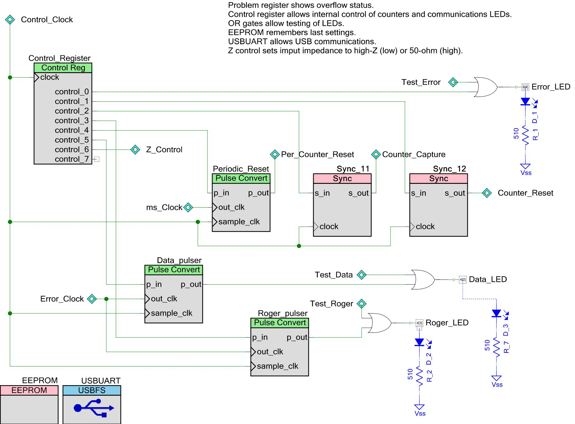
These pulse-shaping networks generate 20ns edge-triggered pulses for the rest of the circuit. They should work for just about any positive input pulse shape, and trigger at a voltage set via software. The Z inputs (open drain, driven low) allow switchable input impedance.
